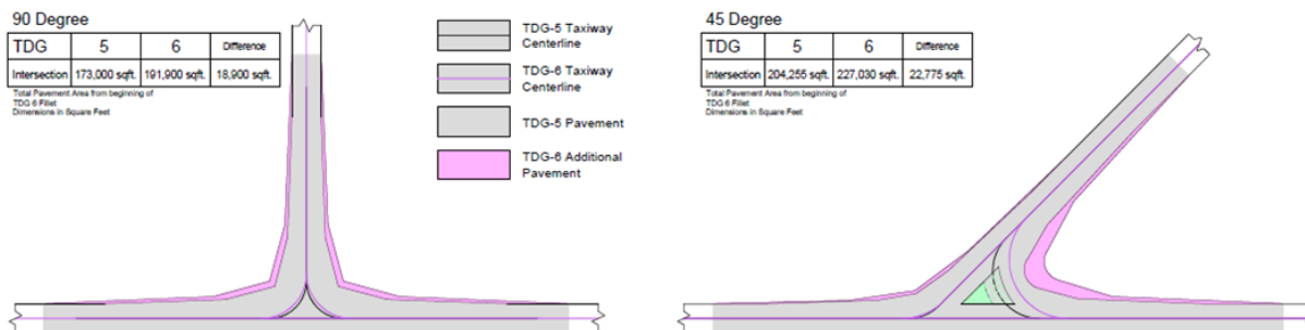
Figure 2-2 COMPARISON OF TAXIWAY DESIGN GROUP 5 AND 6 Airport Master Plan Update Detroit Metropolitan Wayne County Airport
